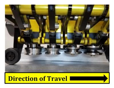
The seamer must be engaged in this manner. Failure to do so will result in panel damage.
